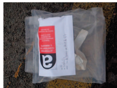
Samples of materials to detect a possible presence of asbestos – © Mairie de Paris, DVD
