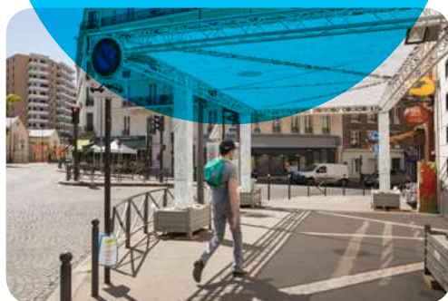
The sun screens, in the form of sails, are also being tested at Place Jeanne d'Arc (13 th - see photo) and on the corner of Avenue de la Porte de Saint Ouen and Rue Huchard (18 th ). Recorded temperatures dropped by 15°C using the system.
